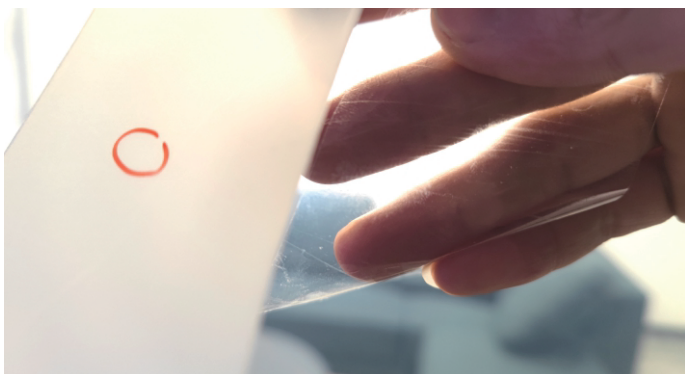
7. How to clean up the foreign objects: Tear off the PDLC film softly, locate the foreign objects, and stick them away with adhesive tapes.
