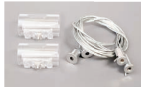
CL-ST-NEON25-360D-Horizontal lifting kit PC tube length: 38mm Length of wire rope: 2m
